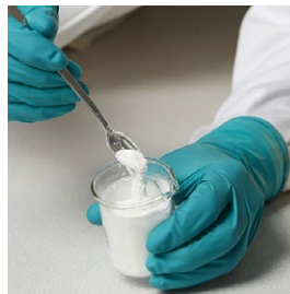
Expancel® DE(T) Dry, expanded microspheres
