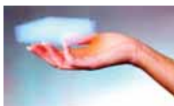
TEOS forms low density insulating aerogels
