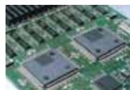
Epoxy-silanes are essential for performance of epoxy resin encapsulants for microchips
