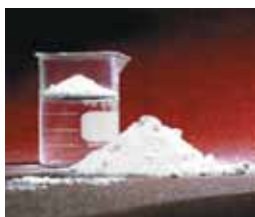
Treatment of fumed silica with hexamethyldisilazane renders it hydrophobic
